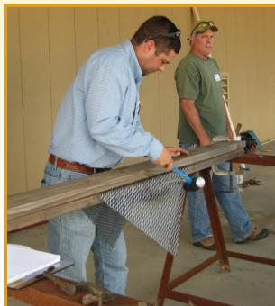
To finalize the shape of the sides, use a hammer to create the proper bends for the ramp.
